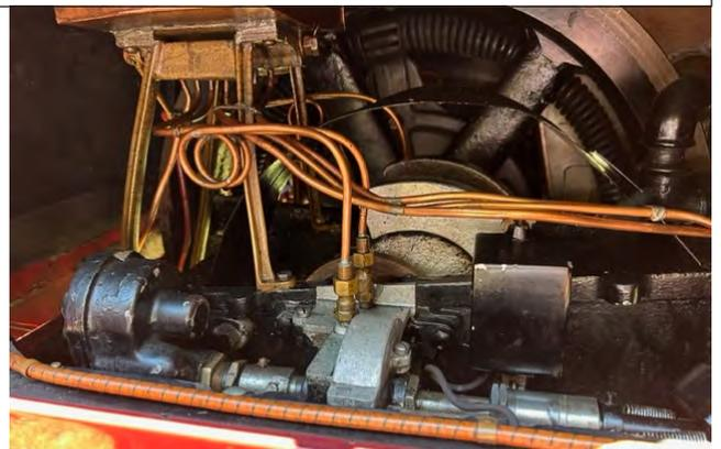
12 Horsepower, Four Stroke, Single Cylinder Packard Engine (Above)
